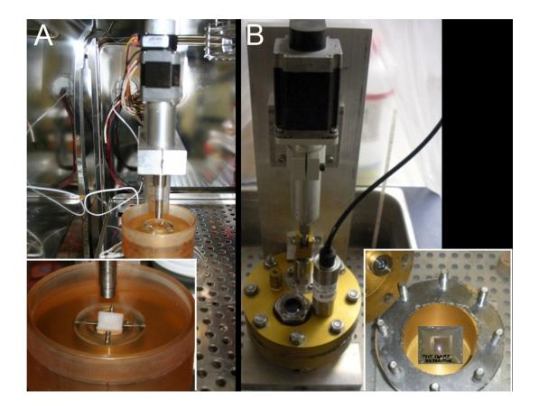
Figure 4. Mechanical loading devices. (A) Device for compressive stress shown in a low oxygen incubator. The inset shows an osteochondral explant submerged in culture medium in the housing under the compression platen. (B) Hydrostatic device shown in a water bath. The inset shows an explant sealed in a plastic bag containing culture medium. The bag is submerged under water in the unit.
